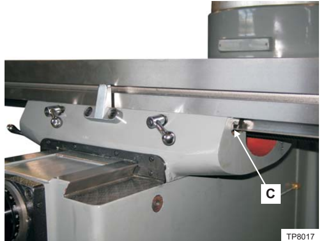
Figure 3.11 - Right Table Gib Adjustment Screw
