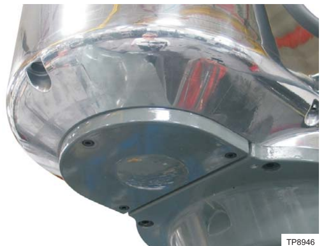
Figure 1.11 - Motor Pulley Cover with Three Screws
