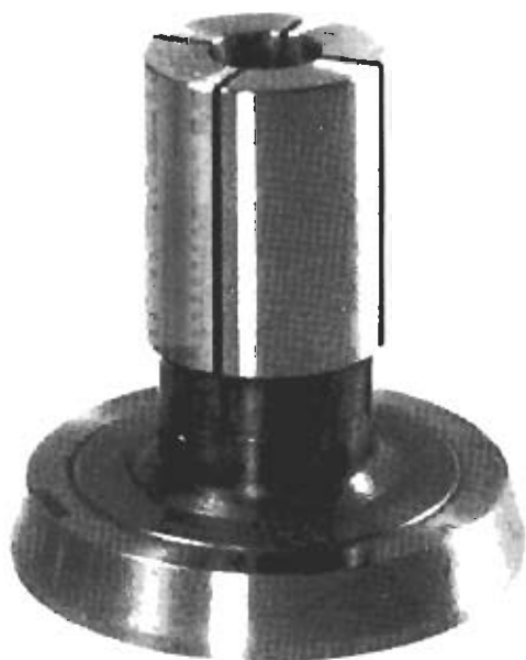
Figure 1 - Hardened and Ground Expanding Collet
